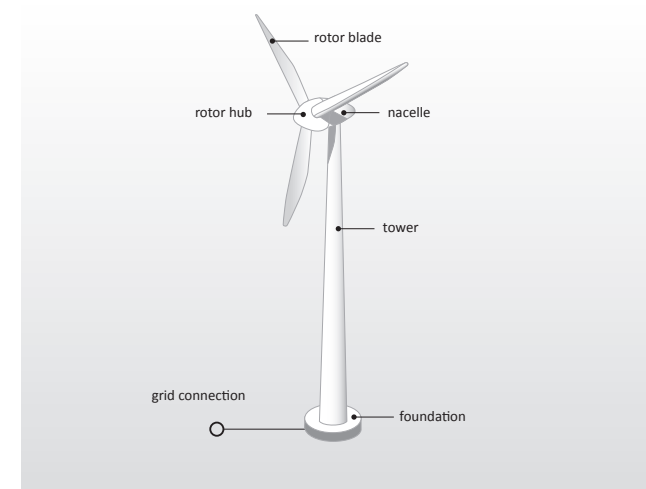
Fig. 3: Components of a wind turbine
