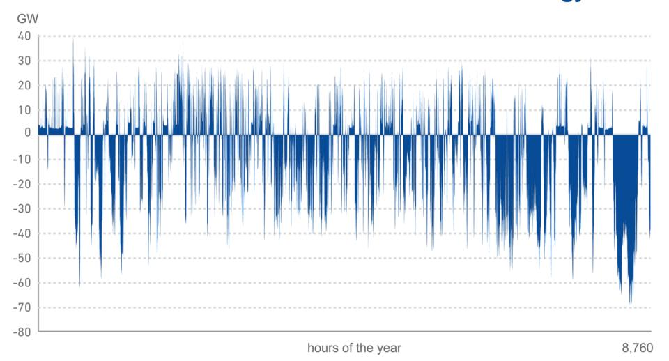
The area below the baseline shows the amount of renewable electricity stored or curtailed (i.e., excess), while the area above shows the need for flexible dispatch.
