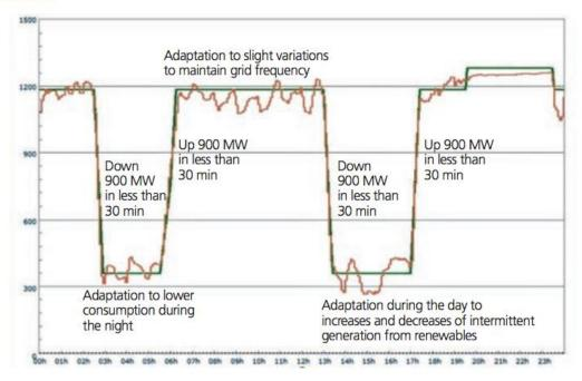
In the latter case, it must be possible to rapidly reduce generation when wind and solar begin to generate their "unavoidable" energy or, conversely, rapidly start up generation when solar or wind production drops. These adjustments are especially important when intermittent generation from renewables is substantial.
